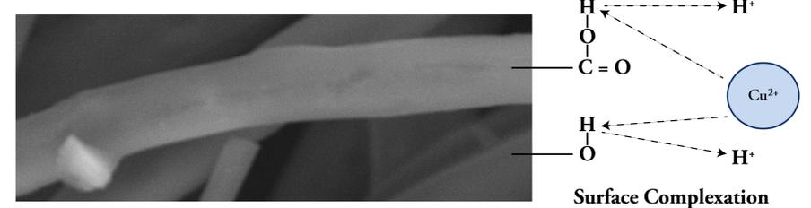
\*Copper metal ions complexate with oxygen-containing groups, ex. hydrogen on carboxylic & hydroxylic groups, assisting chemisorption.
