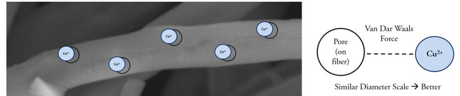
\*LACF contains micro & mesopores, which are on a similar scale with metal ions. In Cu(II)'s case (600pm), micropores on fibers assist the formation of Van Dar Walls force.
